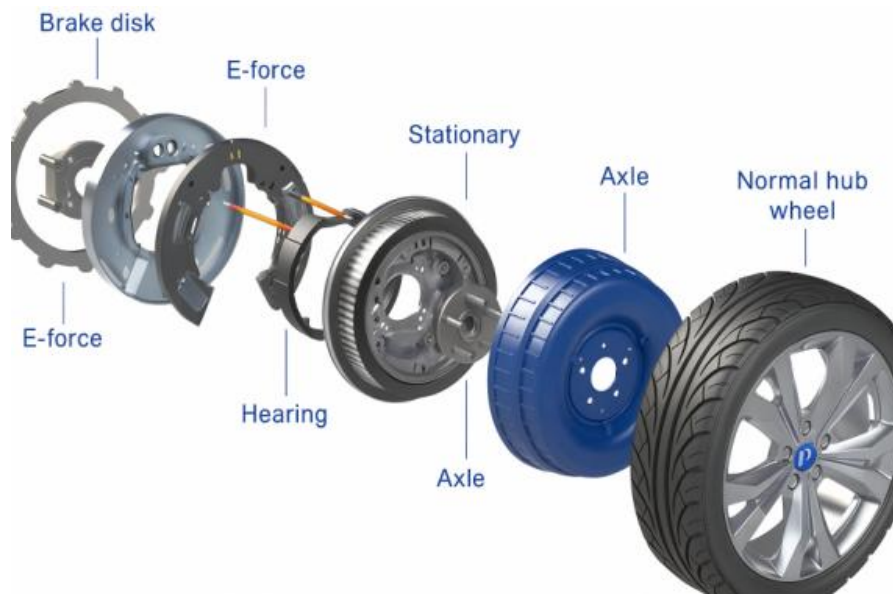
Figure 2. Protean hub motor structure.
